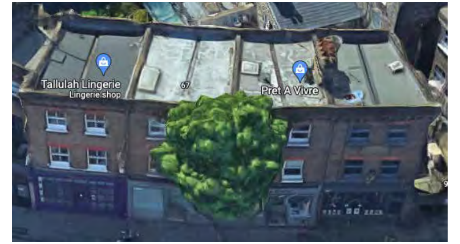
Old Asphalt Flat roof, Harmed Heritage Chimneys & inverted hip roofs removed. Cross Street
